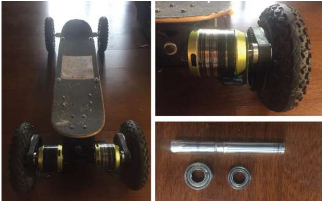
Figure 4.2 Electric skateboard of P19 (Left), Close-up to the engine (Middle), Pieces of the broken engine (right).
