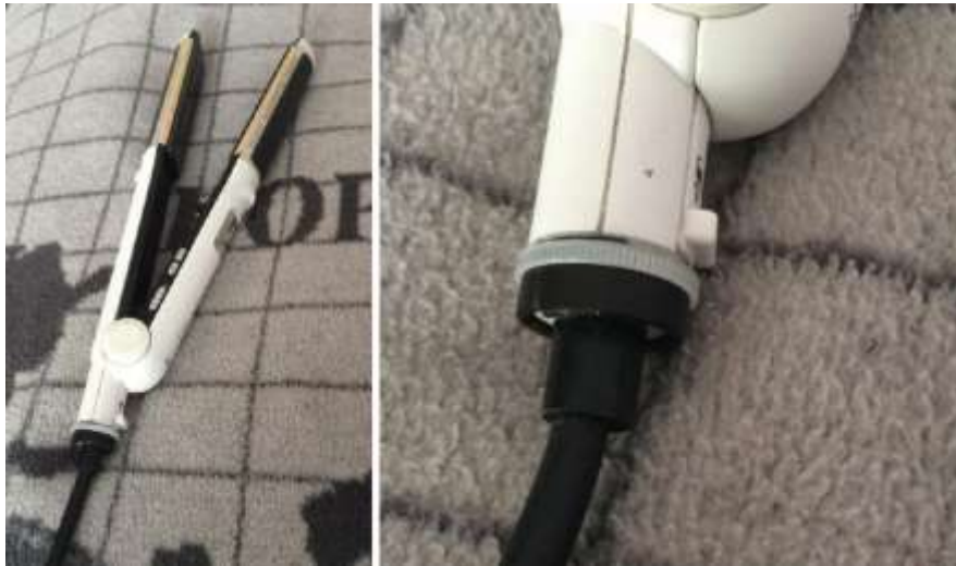
Figure 4.31 Hair straightener repaired by P7 (left) and replaced cord connection (right).
