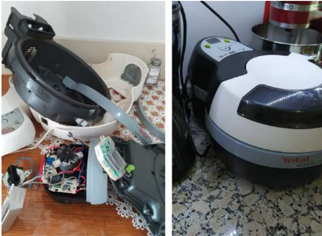
Figure 4.7 Fryer opened up and was ready for repair by P17 (left). Repaired and closed fryer by P17 (right).
