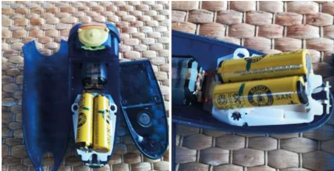
Figure 4.21 Broken shaver that the authorized service couldn't fix is disassembled by P12 and batteries are replaced to make it work again.
