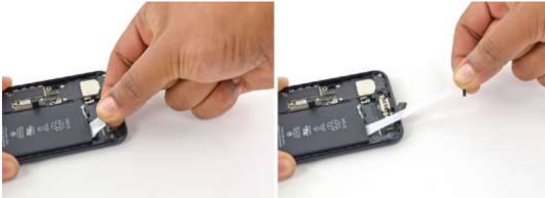
Figure 4.30 Apple's iPhone 7 battery removal by pulling the special tape at a particular speed step by step. (ifixit.com, n.d.).
