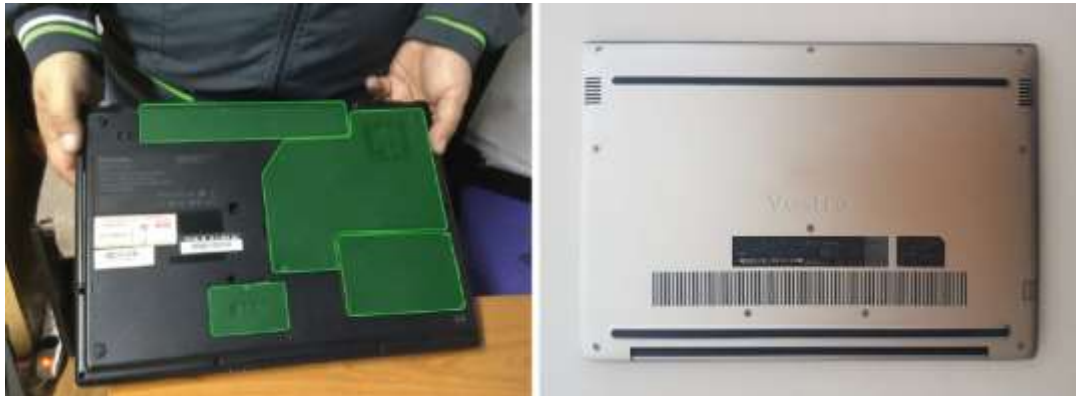
Figure 4.35 P5 shows the separate lids -highlighted with green- for each component of the laptop (left). New versions of the laptop's bottom casing is one-piece (right). Representative photo from author's archive.
