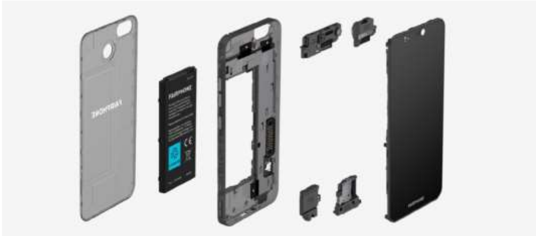
Figure 2.10 Fairphone that has a modular structure with open design sources (Fairphone.com, n.d.).
