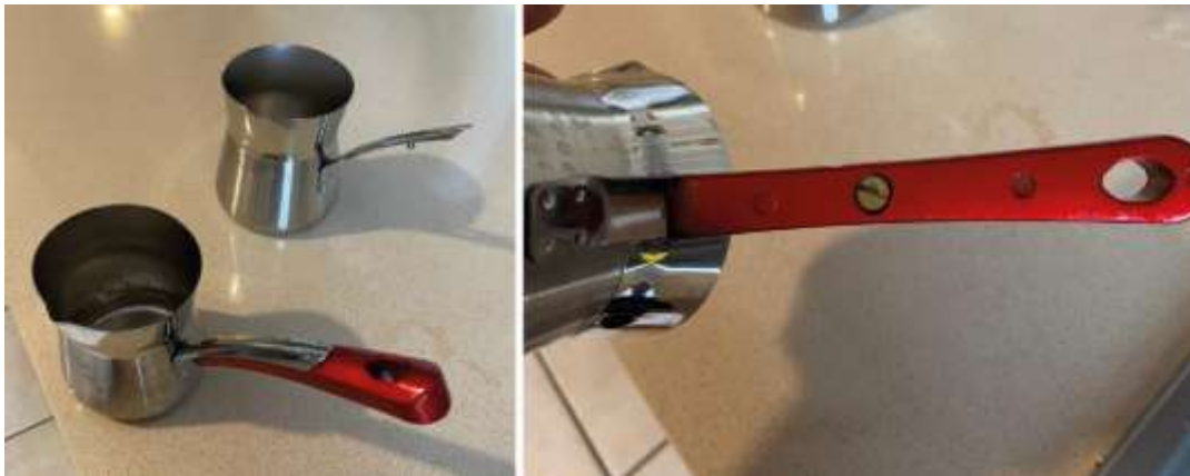
Figure 4.27 Two pieces of the P16's coffee pot set: the solid one is with the red handle while the other's handle is broken (left). The connection detail of the red handle (right).
