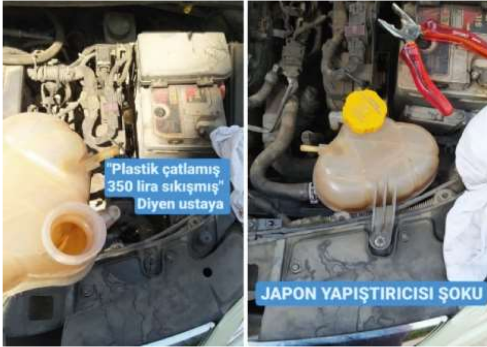
Figure 4.17 Car component P17 fixed with super glue. On the pictures, it is written “Superglue shock”, “for the master who says that the plastic is cracked, 350 TL is stuck”.
