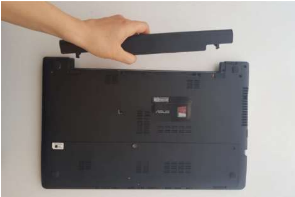
Figure 4.26 2013 model laptop that allows easy battery removal without using any tool. Representative photo from author's archive.
